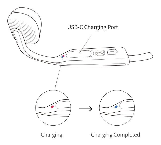
When the headphones are at low battery, there will be a "charge me" prompt and the red light will flash intermittently. Use the corresponding USB-C cable for charging.
